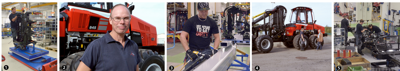
1. Aggregate on air palette for easy circulation. 2. Esbjörn Öberg, Tool Technician, Komatsu Forest. 3. Per Jonsson attaching a linchpin to the hydraulic cylinder that will be located inside the crane boom. 4. Esbjörn and Key Account Manager Dick Sondell from CEJN Norden AB with a Komatsu 845. 5. Production team assembling hydraulic hose and mechanics for a tip-up ladder.
