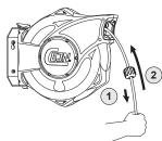
To unlock the cable when you have finished using it, (1) simply pull it out a short distance and listen for the latch to stop "clicking".
