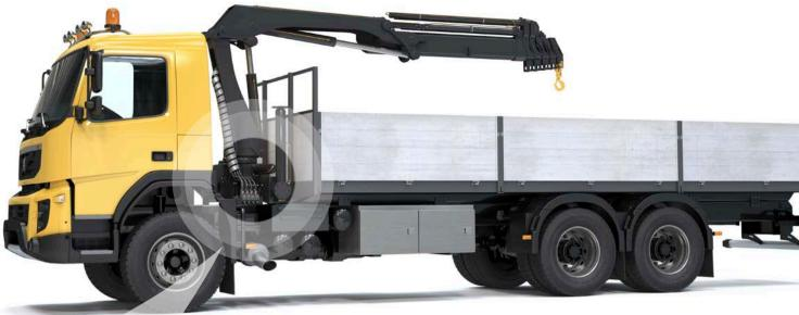
**WHEN IT COMES TO APPLICATIONS WITH EXTREME HOSE MOVEMENT**, the obvious solution is the WEO Swivel. A truck-mounted crane causes the hoses on the valve blocks to twist and rotate in a way that causes them to wear out. When using the WEO swivel, the hoses can move freely and self-align, with 360-degree rotation under full working pressure. The result is longer hose service life and fewer claims.
