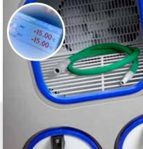
CEJN test area: the hose kits go through stringent tests such as exposure to extreme temperatures.
